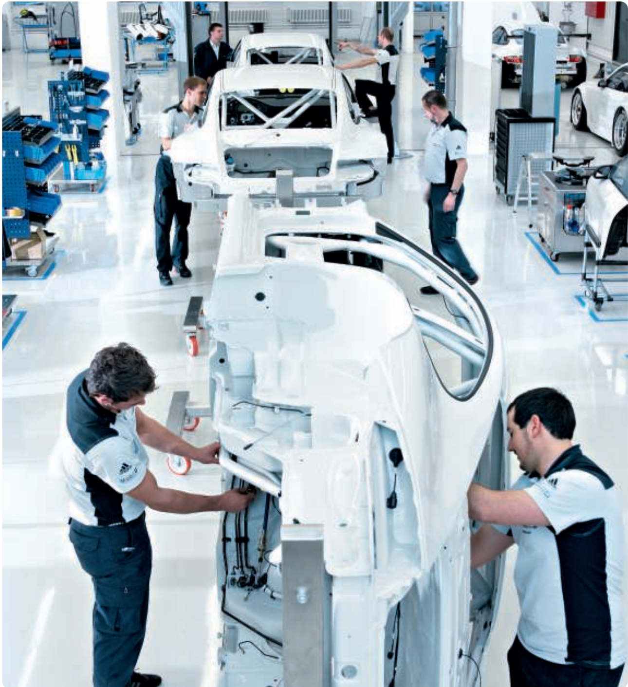
Production-model racing Porsche style: Clarity, order picking trolleys and the pull principle characterise assembly within the factory
