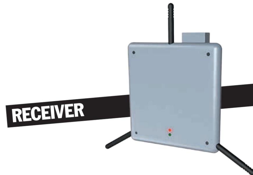
Antennas in the stadium track ball possession, passes, crosses, and shots on goal. They also register performance data such as the height of jumps, the number of steps, the miles run, and speed. The RedFIR system from the Fraunhofer Institute for Integrated Circuits (IIS) uses as many as twelve receivers to gather around 50,000 pieces of data per second. This data is then processed by the SAP HANA platform.
