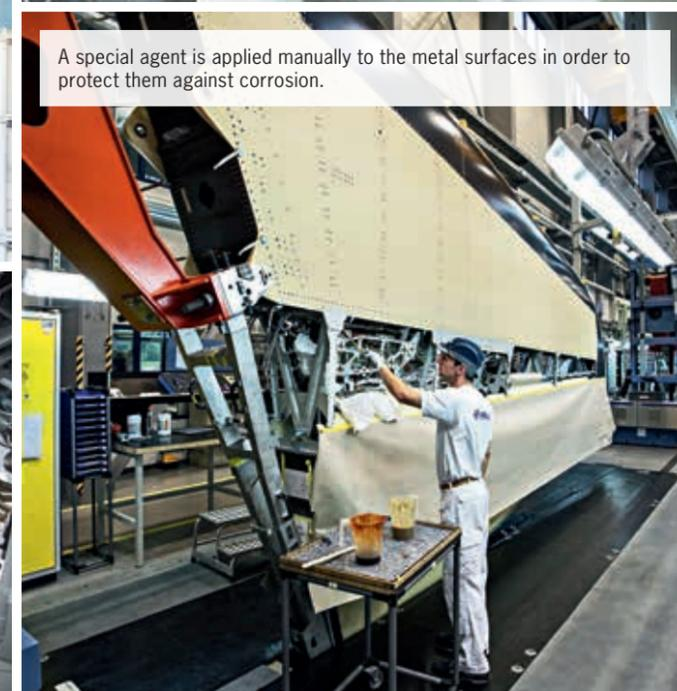
A special agent is applied manually to the metal surfaces in order to protect them against corrosion.
