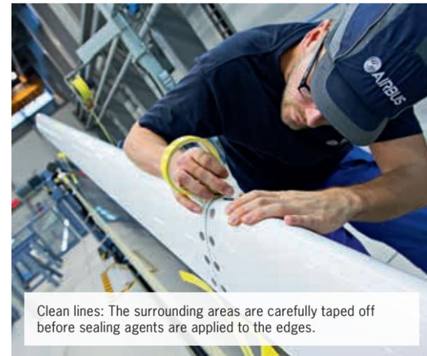
Clean lines: The surrounding areas are carefully taped off before sealing agents are applied to the edges.
