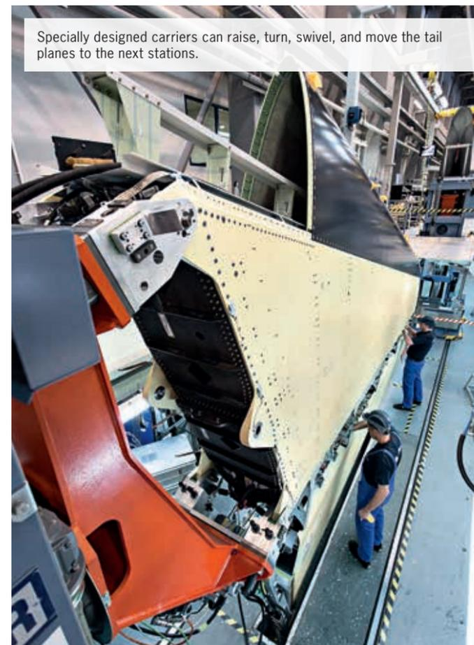
Specially designed carriers can raise, turn, swivel, and move the tail planes to the next stations.
