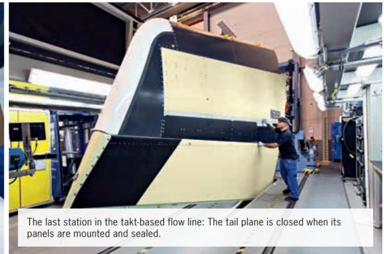
The last station in the takt-based flow line: The tail plane is closed when its panels are mounted and sealed.
