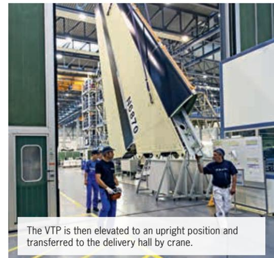
The VTP is then elevated to an upright position and transferred to the delivery hall by crane.
