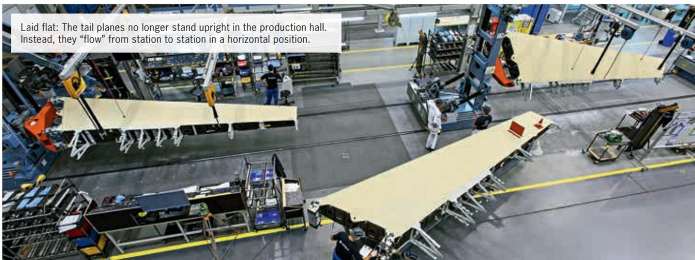
Laid flat: The tail planes no longer stand upright in the production hall. Instead, they “flow” from station to station in a horizontal position.
