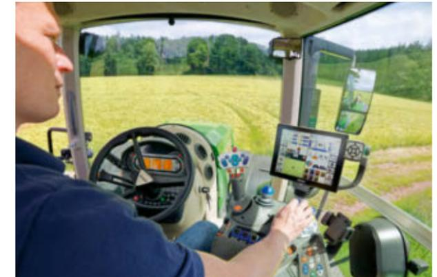
on-board telematics register all data in real time and send various types of information—for example, crop protection agent amounts—straight to the office for the required documentation. I spent the majority of my time in the cabin, which reminded me of an aviation control tower—complete with displays on the screen and tablet just in case I had to intervene in an emergency.
