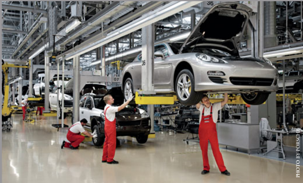
One after the other: The Panamera and Cayenne are assembled in a model mix at the Leipzig plant
