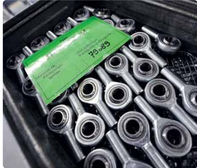
Pivot head with housing – the different sizes and quantities can be produced in real time and finished for the customer
