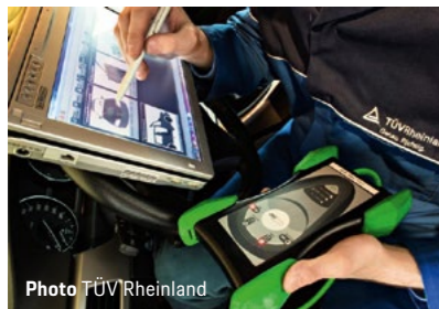
New cars in Germany need to pass their first TÜV inspection within three years, and then every two years after that. TÜV Rheinland inspectors connect an adaptor to the cars' on-board diagnosis interface. That lets them access vehicle data on their laptop, smartphone, or tablet and compare them with those in a central database.
