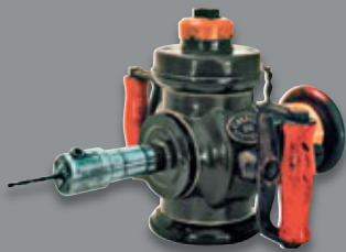
The world's first electrical hand-held drilling machine weighed 7.5 kilos and had a bore diameter of 4 mm
