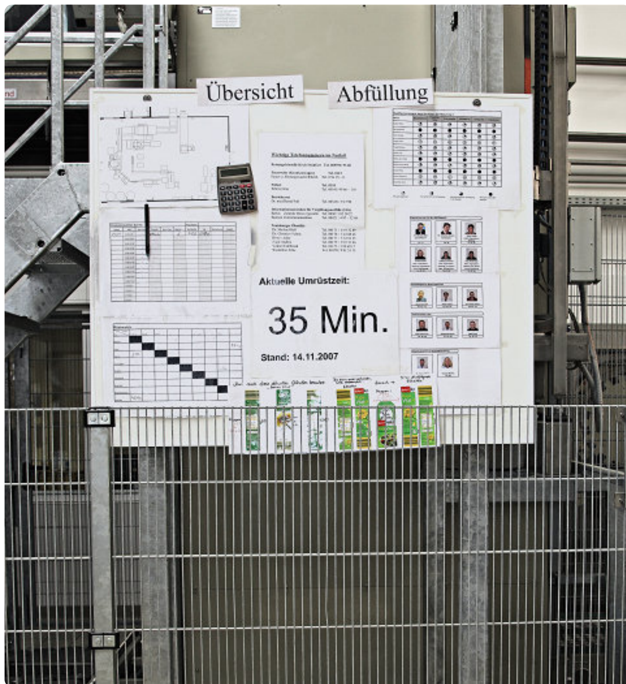
Split time as incentive: The set-up time of 35 minutes has now been cut to 30
