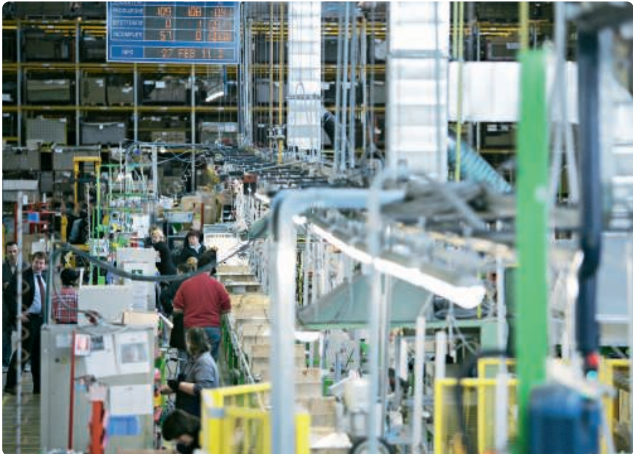
“Just in time” principles in cooker assembly: The work is taking place on the left while the parts ordered from the supermarket can be seen on the right
