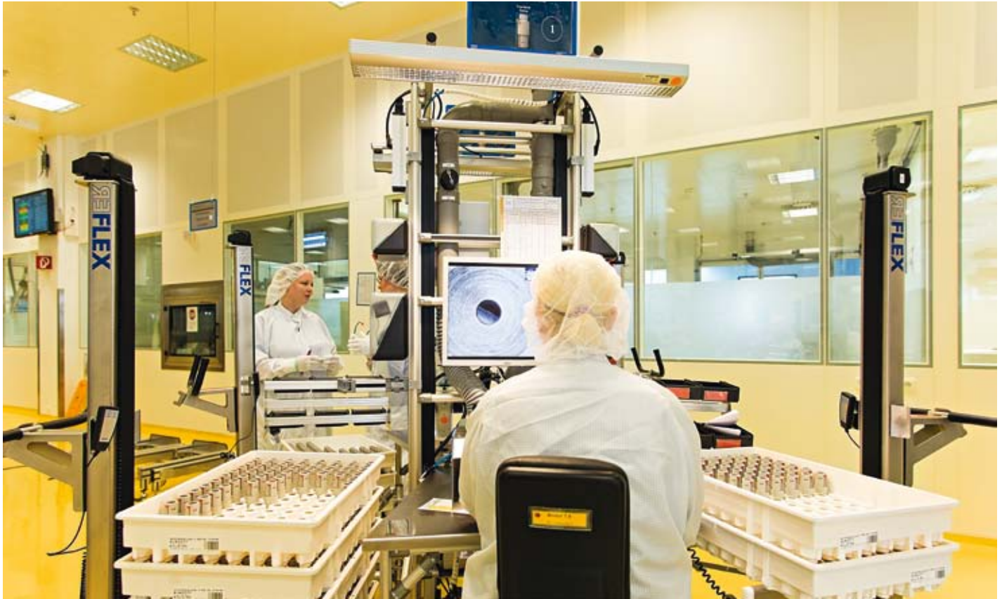
The final production stage combines the different modules and assemblies into the finished RespiMat® inhaler.
